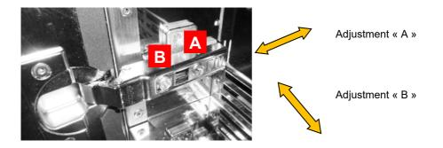
The door is correctly adjusted when the insulating foam presses properly along the whole perimeter and the upper edge of the door has a gap of maximum 2-3mm.
