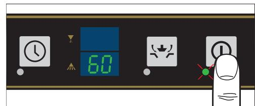
↳ During the filling and heating processes, the button LED flashes. This process can take several minutes.
