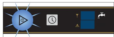
As soon as the machine is ready for operation, the ON/OFF button illuminates green and the fill symbol goes out.
