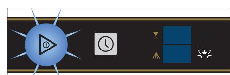
When the drain process is complete, the machine switches off automatically and the key illumination goes out.
