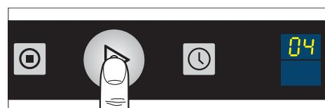
The cycle number is always shown as a 6-place sequence of numbers. First the first 2 places appear on the bottom display on a rolling basis. "1-" appears on the display at the top.
