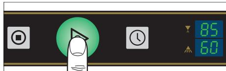
When draining is complete, the machine switches off automatically and the button illumination goes out
