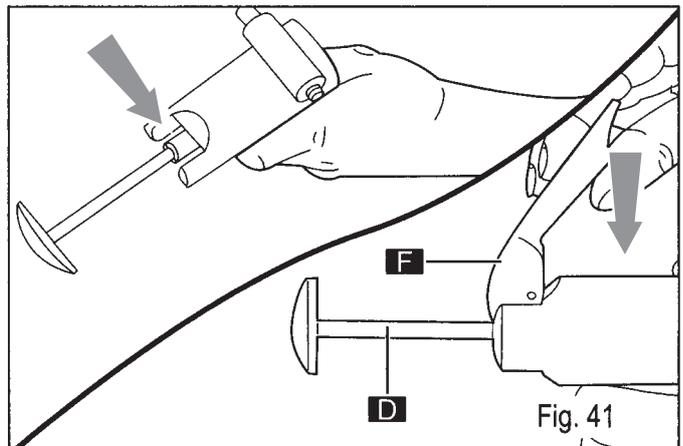
insert the mixer auger into its seating;
