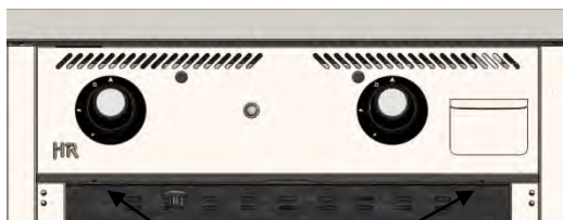
DESMONTAR PANEL (A)
