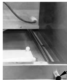
Dripping trough for condensed water
